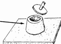
To make the **closed latrine**, the slab should be placed over a round hole in the ground. Dig the hole a little less than 1 meter across and between 1 and 2 meters deep. To be safe, the latrine should be at least 20 meters from all houses, wells, springs, rivers, or streams. If it is anywhere near where people go for water, be sure to put the latrine **downstream**.
