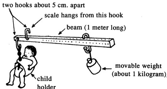
Weight is correct when beam stays horizontal.
