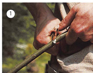
Breaking: Make a series of small cuts around the work piece to weaken it, then snap it in half.
