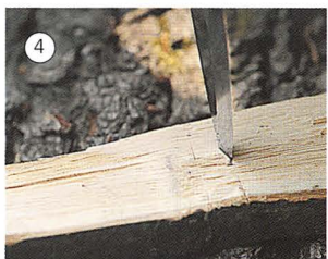
Using lines and estimation repeat hole making, until holes meet in the middle
