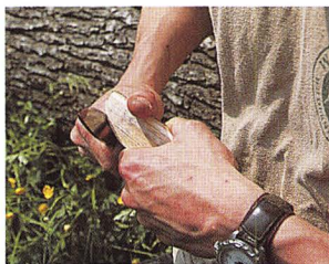
Shaping: By pivoting around the thumb.
