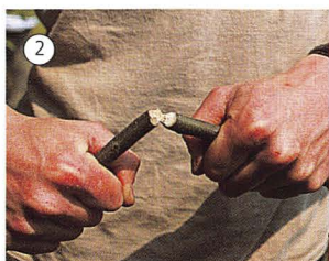
Breaking: Make a series of small cuts around the work piece to weaken it, then snap it in half.
